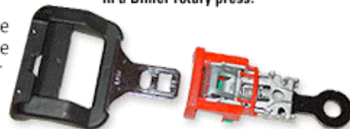
This part was stamped on a 200-ton press and then further processed in a Bihler rotary press.
