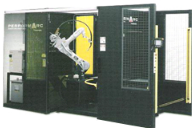
Our 6-axis articulated robotic welder utilizes a servo-controlled, high-speed 60-inch turntable.
